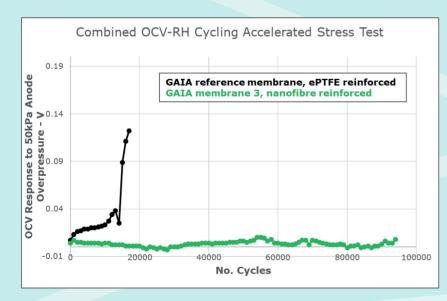
An MEA comprising a thermostable nanofibre reinforced perfluorosulfonic acid membrane of 15 µm thickness has withstood an exceptional 100,000 accelerated stress test cycles of combined open circuit voltage hold and relative humidity cycling at 90 °C, considerably exceeding the target 20,000 AST cycles for light duty vehicles.
